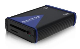
**Omni***Drive USB CF/SD* is an external drive for Compact Flash cards and for SD cards. Using an appropriate adapter, you can also read/write micro-SD Cards.
